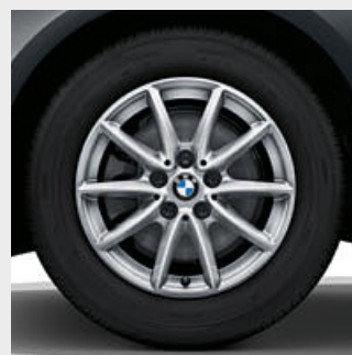
■ 16" light alloy wheels V-spoke style 471* in Reflex Silver, wheel size 7J x 16, with 205/60 R16 tyres.
